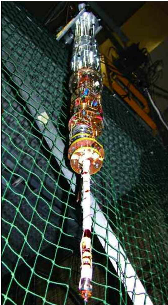
Figure 4. This dilution refrigerator at Los Alamos National Laboratory is able to cool a sample to 20 mK (1/50 of a degree above absolute zero, or roughly -460°F). The blue object in the background is a 20 tesla superconducting magnet, roughly 10 times more powerful than the magnet on a typical magnetic resonance imaging machine.
