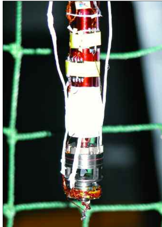
Figure 4. This dilution refrigerator at Los Alamos National Laboratory is able to cool a sample to 20 mK (1/50 of a degree above absolute zero, or roughly -460°F). The blue object in the background is a 20 tesla superconducting magnet, roughly 10 times more powerful than the magnet on a typical magnetic resonance imaging machine.
