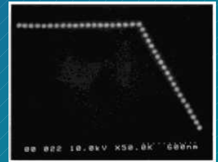
Plasmon wave guide from d~50 nm gold dots.
