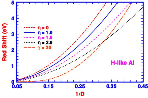
FIG. 2. (Color online) Simulated Lyman- $\alpha$  redshifts of H-like  $\text{Al}^{12+}$  as functions of  $1/D$  with the radius of Debye sphere  $A$  given by  $\gamma = 20$ , and  $\eta = 0, 1.0, 1.5$ , and  $2.0$ , respectively.
