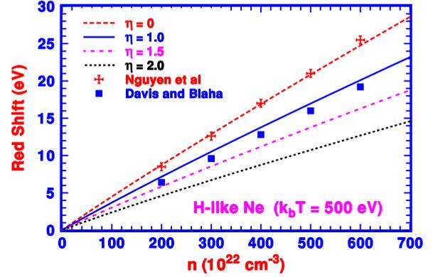
FIG. 4. (Color online) Comparison between our simulated redshifts as a function of density  $n$  at 500 eV of H-like  $\text{Ne}^{9+}$  with results from existing quantum mechanical approaches by Nguyen *et al.* [8] and Davis and Blaha [12].
