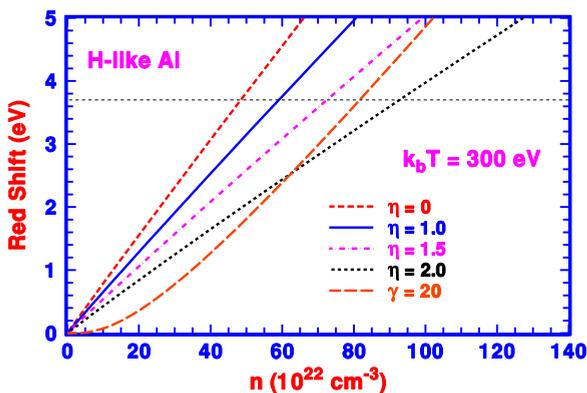
FIG. 3. (Color online) Simulated Lyman- $\alpha$  redshifts of H-like  $\text{Al}^{12+}$  as functions of density  $n$  at 300 eV with the radius of Debye sphere  $A$  given by  $\gamma = 20$ , and  $\eta = 0, 1.0, 1.5$ , and  $2.0$ , respectively.
