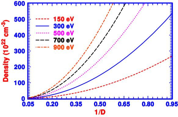
FIG. 1. (Color online) The variation of plasma density  $n$  as a function of  $1/D$  at various electron energies.
